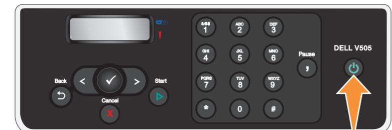
**8 Press the Power button on the operator panel to turn on your printer.**
