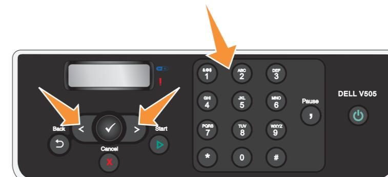
**9 Use the arrow buttons and the keypad to specify your language, country, date, time, fax number, and fax name. Press the Select button (S) to save each setting. If you need to reset the language, hold the Back (B) and Start (S) buttons while turning the power on.**
